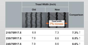
The optimized footprint and an increased tread area improves mileage and prevents separation.
